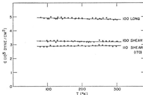
FIG. 2. Sound velocity in  $Mg_2Sn$ : [100] and [110] directions.
