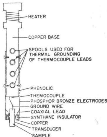
FIG. 1. Sample holder for sound velocity measurements.
